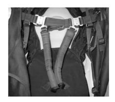
The safety has also been improved by optimising the position of the back protection; the rear pocket has been moved upwards, offering protection for the pilot in case he accidentally falls on his back.
